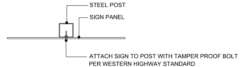
C ATTACHMENT DETAIL - PLAN SECTION
